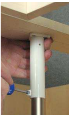
3. Fix the upper bearing
