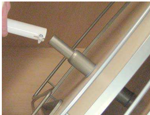
4. Put the upper bearing cover on the axle
