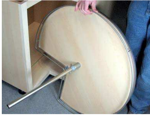
2. Put the bottom shelf on the axle
