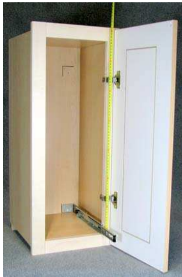
5. Mark the height of the frame in the carcass
