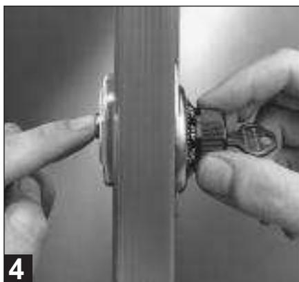
**4** With other hand, turn dial right to number 48. Do not turn dial more than two numbers with button depressed. Then release push-button.
