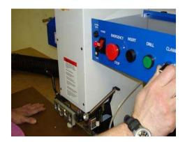
19.) Drill hole pattern. Press the DRILL/IN-SERT SAFETY BUTTON with the left hand and hold while pressing the DRILL button on the control panel with the right. The machine will drill the hole pattern.
