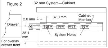
3. Use only the 32 mm system holes or the wood screw holes located at the tip of the breathing tabs. Do not use any other holes on the cabinet member for mounting (Figure 3).
