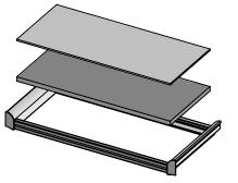
CUT AND PLACE A 3/4 INCH BASE INTO THE FRAME, THEN ADD THE FABRIC WRAPPED BASE ON TOP.
