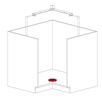
Please refer to your fitting specification document, if you have to use the 3mm spacers. If the spacers are specified, please mount them between the top mounting bracket and the side wall. This assures the correct position of the upper pole bearing.
