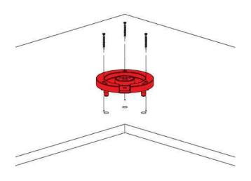
If cabinet has a top, proceed with 4.Installation of fitting, (page 6). (--> mainly face frame cabinets)
