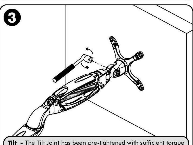
**Tilt** - The Tilt Joint has been pre-tightened with sufficient torque to ensure you can adjust your screen to an appropriate angle. If your screen droops, additional torque can be applied by using an 8mm socket wrench applied to the locking nut on the left hand side of the arm.
