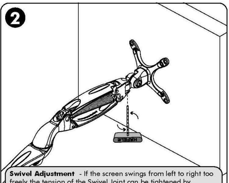
Swivel Adjustment - If the screen swings from left to right too freely the tension of the Swivel Joint can be tightened by applying the T-Bar Hafele Key to the domed nut on the underside and turning it anti-clockwise until sufficient tension is applied.
