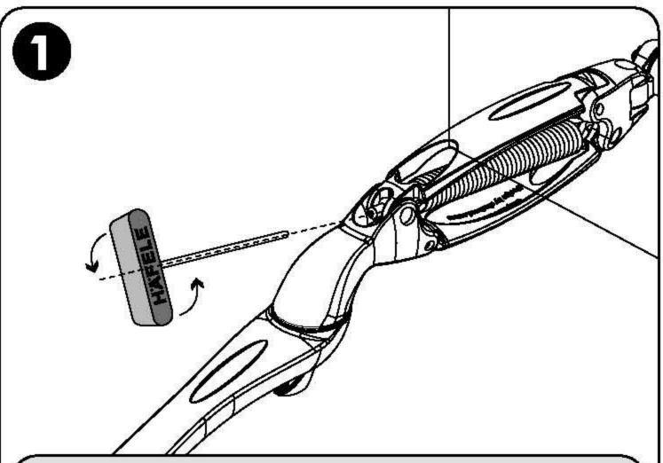
**Spring Adjustment** - The spring tension needs to be calibrated to the weight of the LCD Screen. If the screen rises of its own accord the tension is too high. Using the T-Bar Hafele key turn the screw anti-clockwise. If the screen droops the tension is too low. Using the T-Bar Hafele Key turn the screw clockwise.
