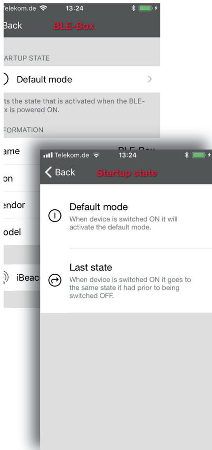
With the Startup State setting you can set the device to either go to default light level or to the last state when the device is switched on. With the Last state setting the device will go to same dimming level and colour as it was when the device was switched off. You can also determine a minimum level for the Last state setting. Then the device will always go to at least the minimum level when turned on.
