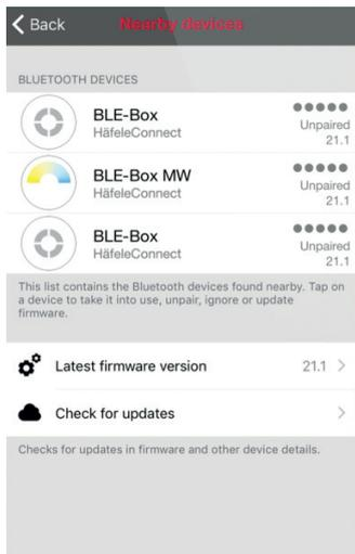
When you tap on the device you will see the options that are available. You can add to an existing or new network, change the profile of the device or ignore the device. Or, if available, you can update the firmware.
