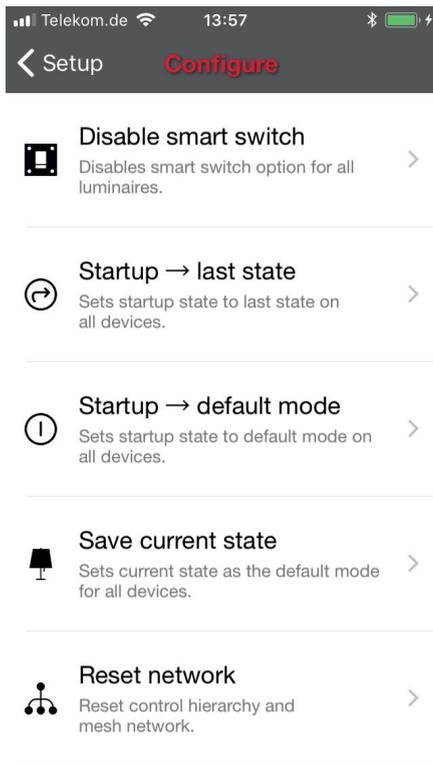
It is possible to configure all devices in a network by selecting Configure all devices under Network Setup.
