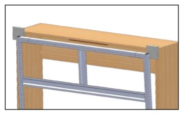
Install the permanent stopper on the inside top of the cabinet where it will allow for the door to close flush to the front of the cabinet.
