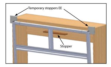
Install temporary stoppers **EE** onto the top corners of the bed cabinet.
