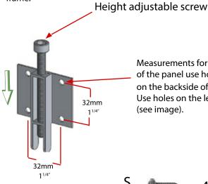
Measurements for the right side of the panel use holes on the right on the backside of the doors. Use holes on the left for the left side.
