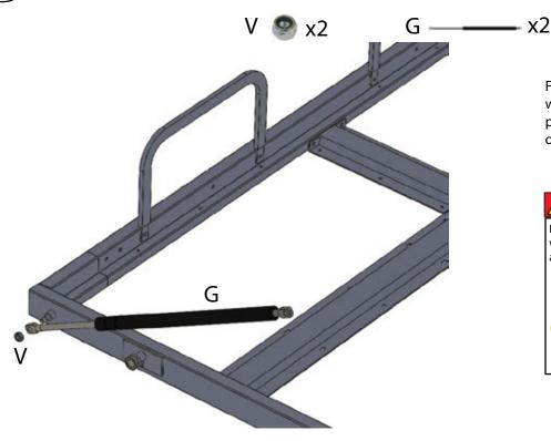
Follow the arrows on the piston indicating which side is "up" in order to install the piston properly and ensure the longevity and proper operation of the piston.
