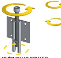
Note that ends are rounded so that doors can slide left - right for a better adjustment.
