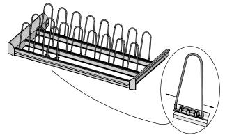
STEP 1: SPREAD SHOE HOLDERS AND INSERT THE ENDS INTO BOTH SIDES OF THE CLIPS LOCATED INSIDE THE CROSS-BARS. ENSURE HOLDERS ARE ANGLED TOWARDS THE REAR OF THE FRAME.
