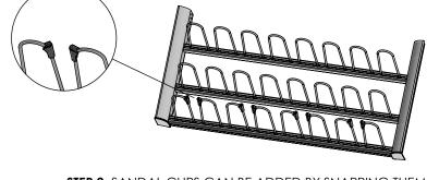
**STEP 2:** SANDAL CLIPS CAN BE ADDED BY SNAPPING THEM ONTO THE SHOE HOLDERS.
