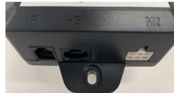
Plug the other Column Into Port M2 - HS Port is for the Switch - F Port is not used
